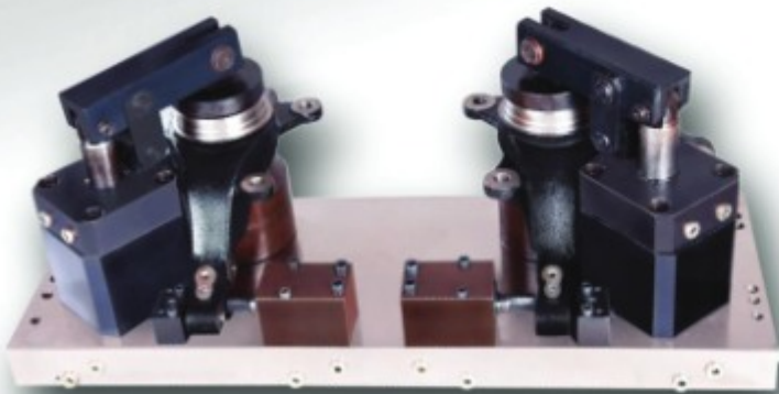
▲ Two Stations in One Fixture
